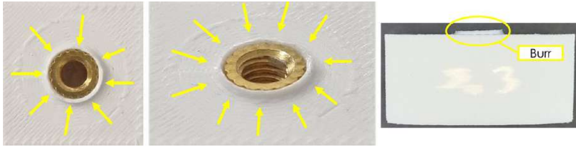
Figure 8. Circumferential burr formation at the hole edge
