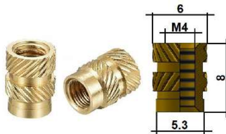
Figure 2. Threaded metal insert geometry and dimensions
