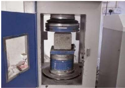
Compressive strength testing machine showing cube subjected to loading
